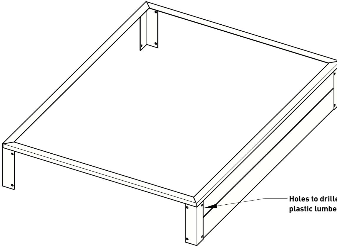
Holes to drilled directly into the plastic lumber and use a lag screw to tighten
